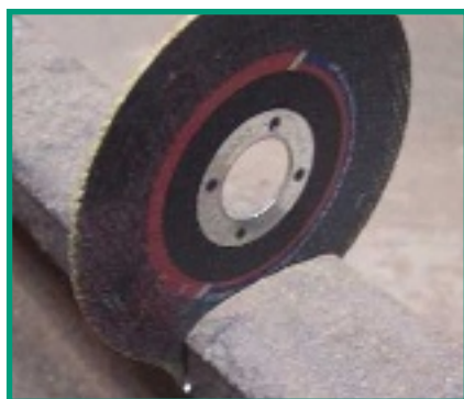
Thick Cut in Train Rail
