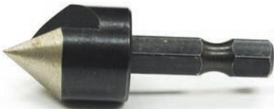
The Quick Change series of tool steel countersinks is suitable for deburring, chamfering, or countersinking the mouth of a hole in metal, plastic or wood. Each is made of fully hardened 5/8" diameter tool steel and has a single flute. These fit straight into the Quick Change chuck without an adapter. The 82° countersink is used for most common tapping screws, wood screws and floor board screws. The 100° countersink is used for certain aviation rivets and other specialty fasteners.
