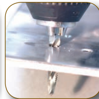
Push deburring collet into hole lightly.
