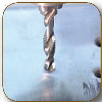
Drill hole using recommended RPM and medium pressure.
